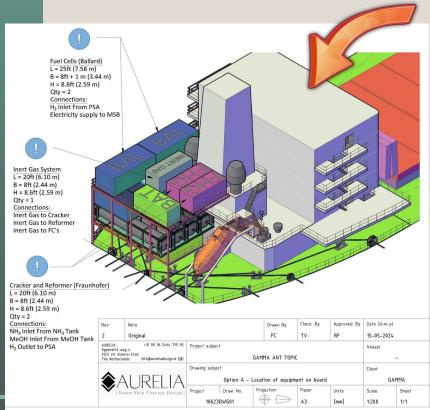
On the second level are located the new technology containers for reforming methanol and cracking ammonia. The obtained hydrogen will be purified in PSA unit and used for the fuel cell, also located on the top level of the new platform.
